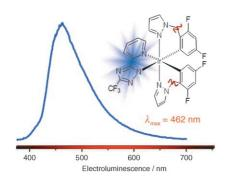
**True blue**: The nonconjugated nature of a methylene spacer interrupts the  $\pi$  conjugation of the cyclometalated ligands, which lowers the  $\pi$  orbital energies and destabilizes the respective  $\pi^*$  orbitals. Incorporation of a third chelating chromophore with a blue-light energy gap induces true-blue-light emission at room temperature (see figure).
